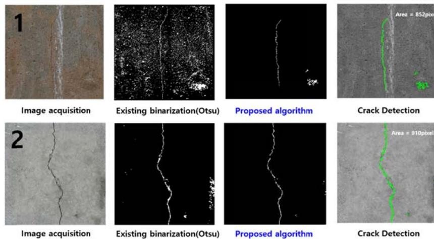
Fig. 6 Results of crack detection in the field test
