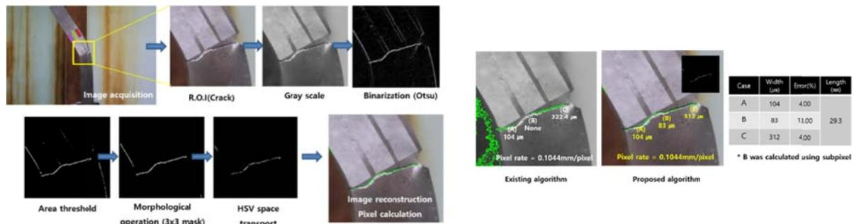
Fig. 3 Steps for application of crack detection algorithm
