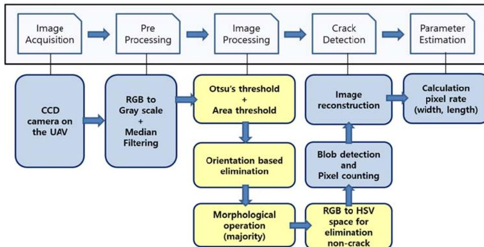
Fig. 1 The proposed crack diagnosis algorithm
