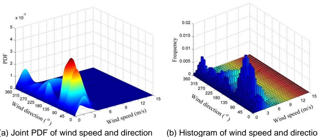
Fig.1 Joint distribution of wind speed and direction by proposed approach
