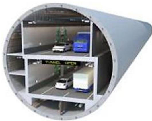
Fig. 1 Structure of double-deck tunnel
