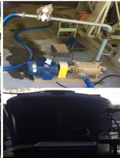
Fig. 4 Pump station and water tank (5ton)
