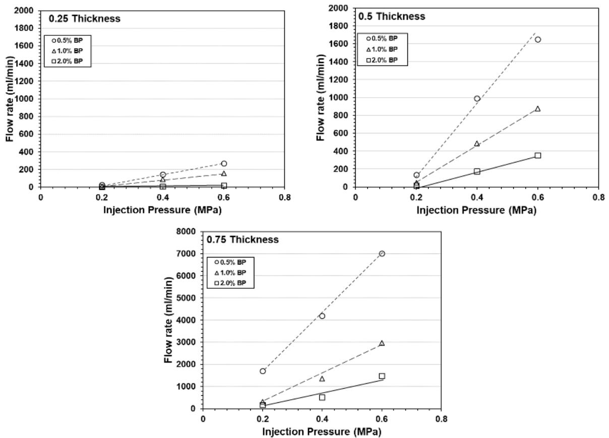
Fig. 3 Injection performance of Xanthan gum in laminar flow
