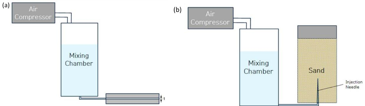
Fig. 2 Experimental Design of (a) laminar flow (b) into soil mass
