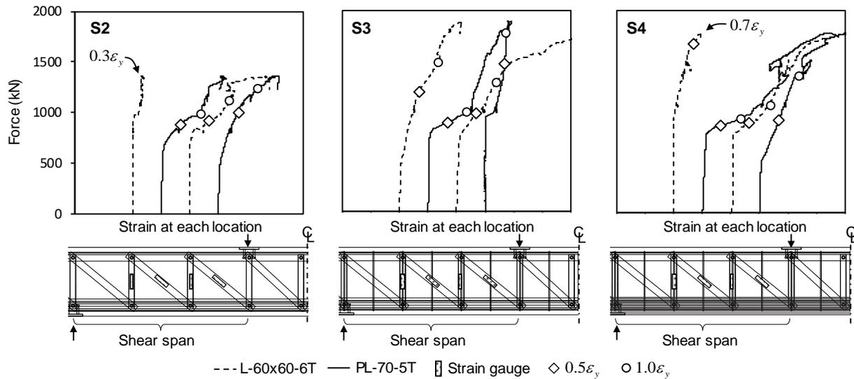
Fig. 3 Strain gauge of web truss
