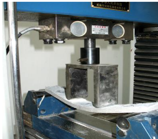
Fig. 3 Four-point bending test of ECC
