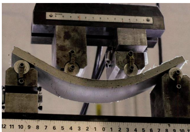
Fig. 1 ECC deformed by bending
