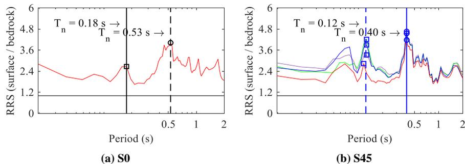
Fig. 3 Ratio of response spectrum: (a) S0; (b) S45
