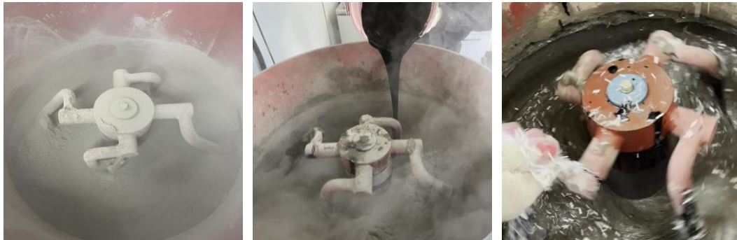
Fig. 1 Mixing CNT dispersed aqueous solution and PVA fibers
