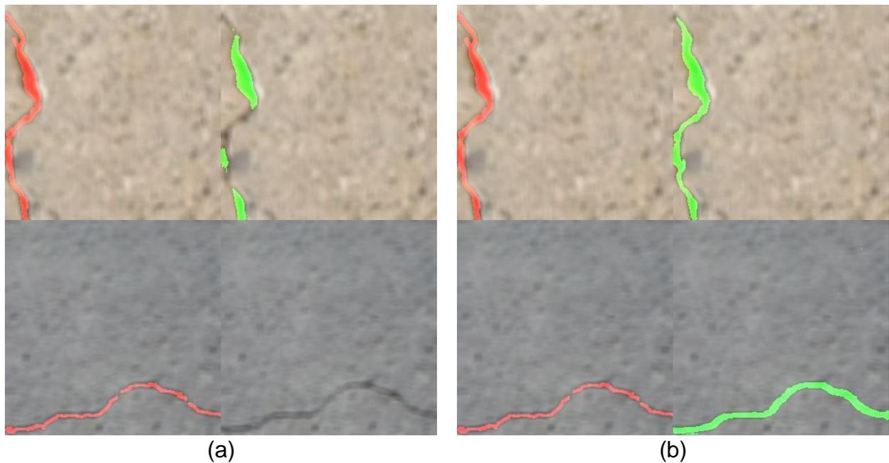
**Fig. 3** Results of crack detection; (a) original, (b) proposed method
