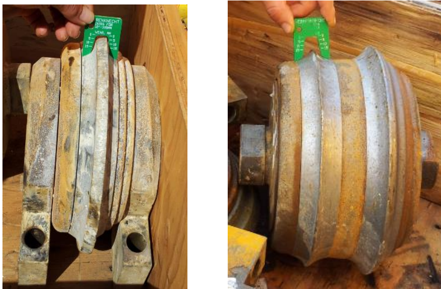
Fig. 14 Difference between a cutter without wear and a cutter with heavy wear
