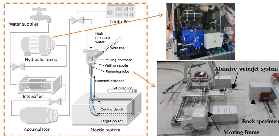
Fig. 2 Experimental setup for abrasive waterjet rock cutting
