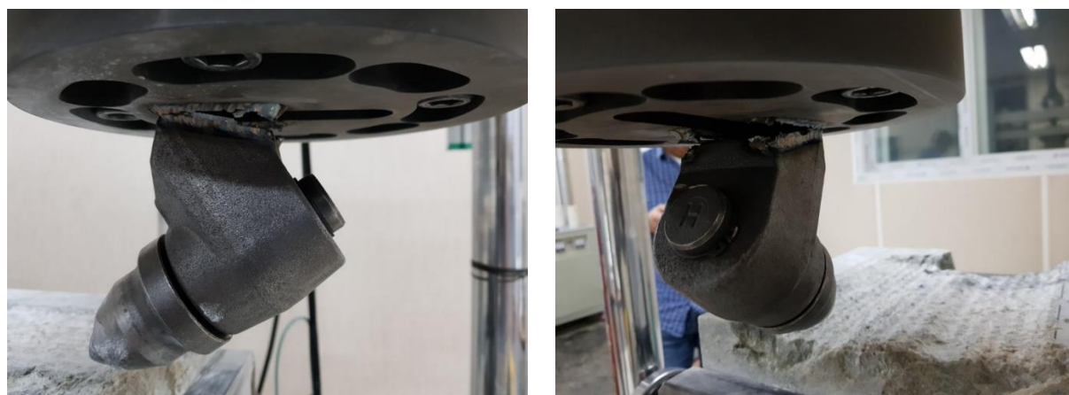
Fig. 7 Tearing in welding part between holder and plate
