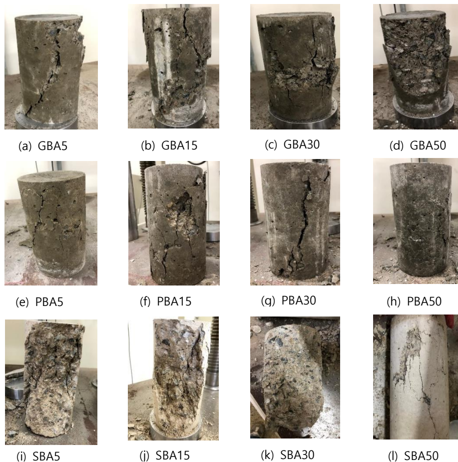
Fig. 5 Failure Mode of Specimen
