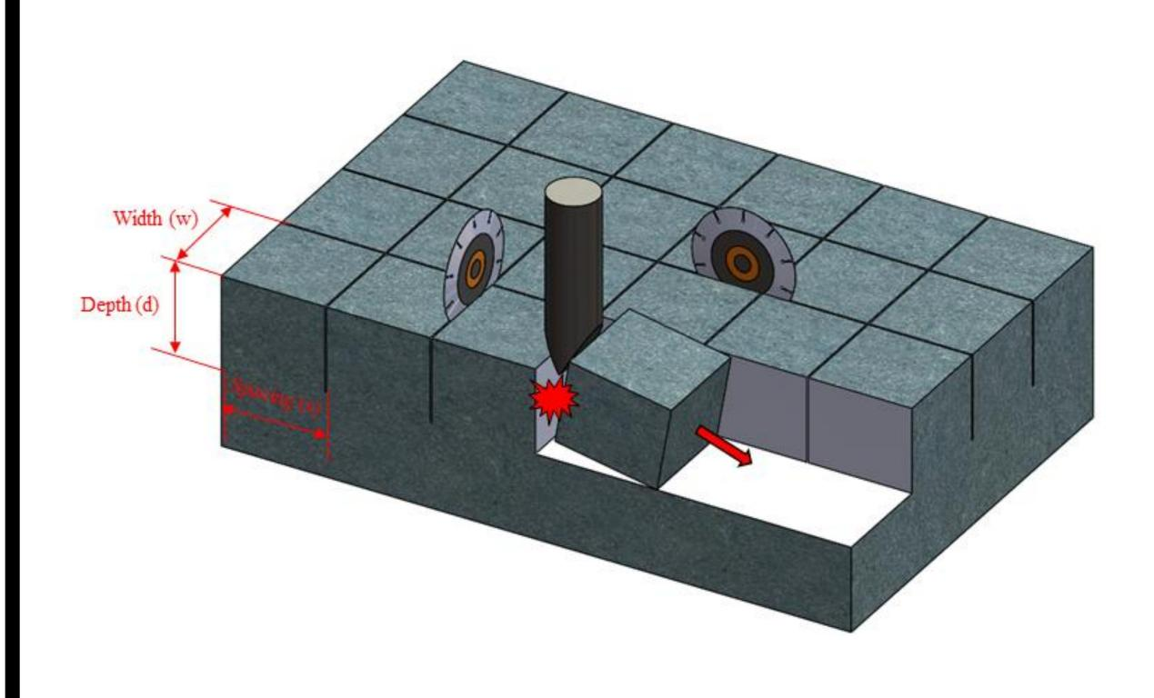
The proposed method is cutting-splitting method which is consisted of two processes: cutting and splitting. First step is rock cutting by a rock saw according to the predesigned dimensions Then, a sharp chisel is percussed into the cutting slot to propagate the tensile crack on the bottom surface of rock mass.
