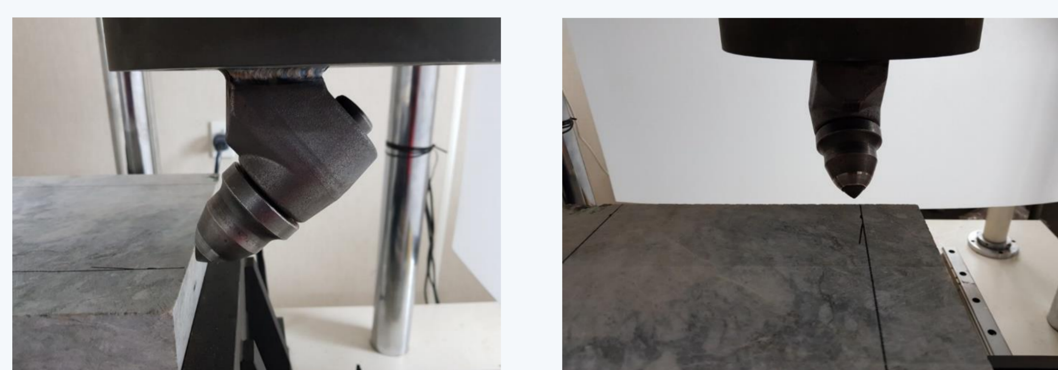
Fig. 1. Experimental set-up of the LCM test
