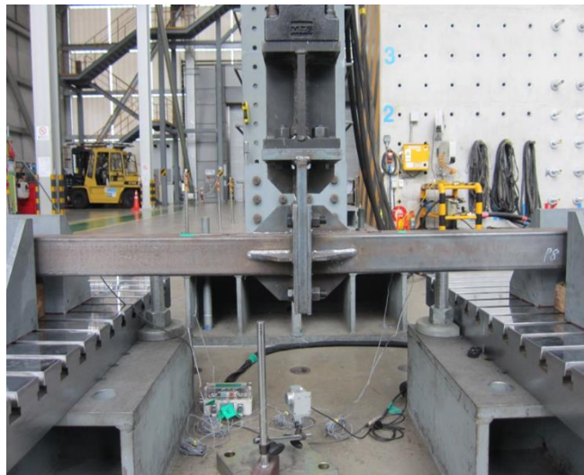
(a) Schematic of experimental apparatus (b) WRR specimen under loading
