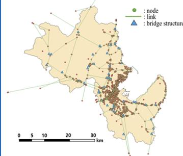
The proposed methodology is applied to an actual bridge transportation network located in Pohang city, Korea (Yoon et al. 2020). The target bridge network consists of 1440 nodes and 3490 links, and bridge components connecting each road network consists of 48 long-span bridges, including highways and national highways.
