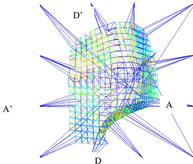
Fig.2 collapsing procedure of the double layer grid due to support loss with an abnormal live load
