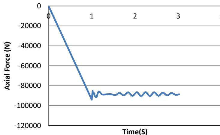
Fig. 1 Axial Force in the Top chord near the removed central pyramid.
