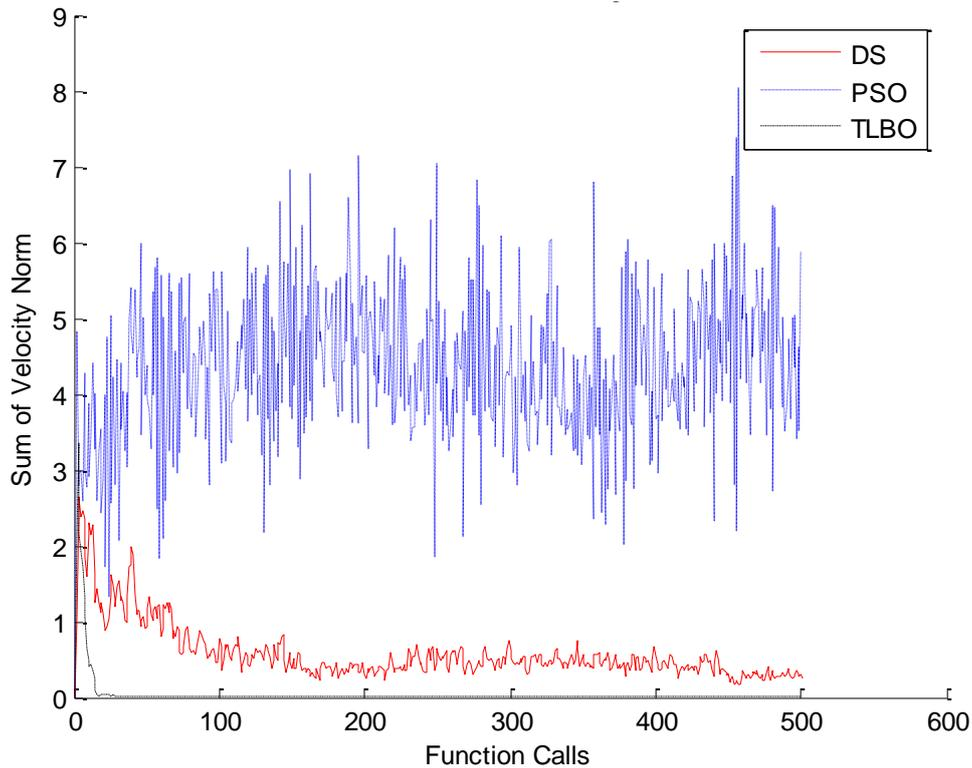
Fig.11 Diversity comparison between PSO, TLBO and DS in the 3-bar truss design
