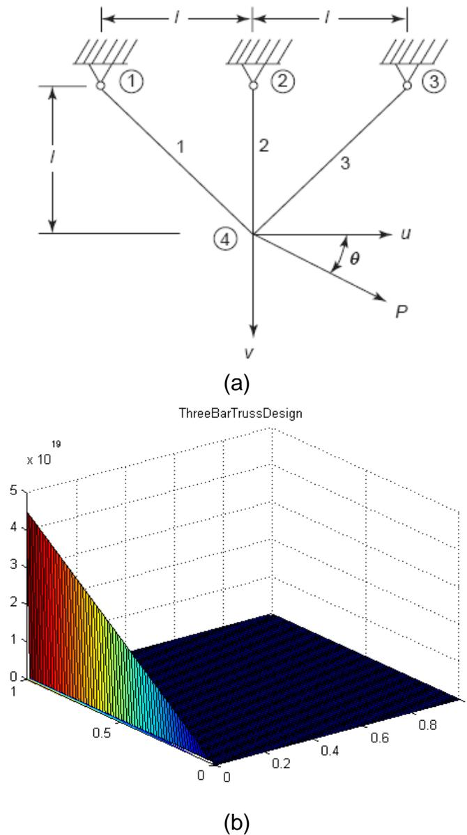
Fig.10 (a) The structural model and (b) design space of the 3-bar truss problem
