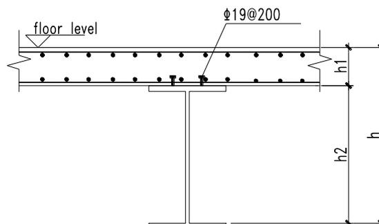
Fig.1 the diagram of the height of composite floor
