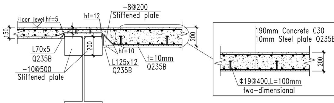
Fig. 5 Section of the composite floor
