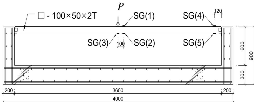
Fig. 2 Elevation of M-F-A50-B and M-F-A80-B
