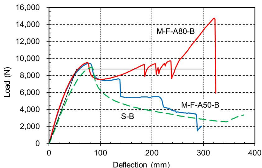
Fig. 4 Load-Deflection depending on support conditions
