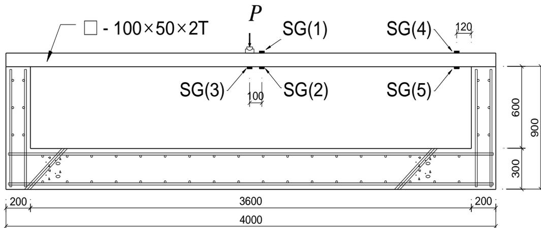
Fig. 1 Elevation of S-B
