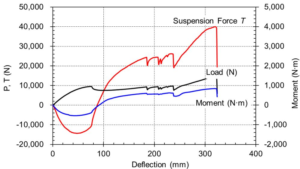
Fig. 5 Tension, Moment and Load of M-F-A80-B
