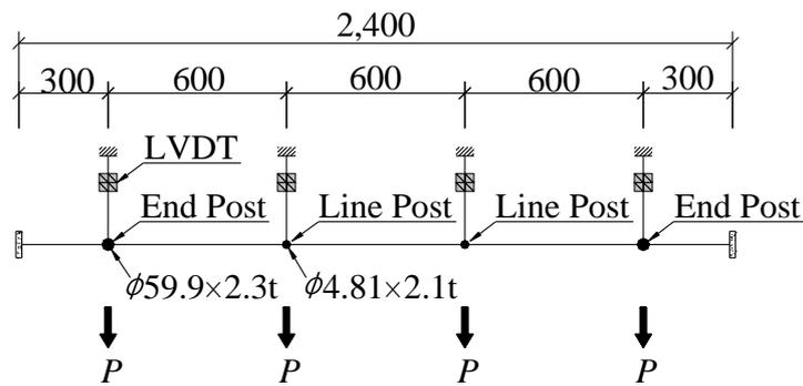
Fig. 1 Floor plan of fence support system
