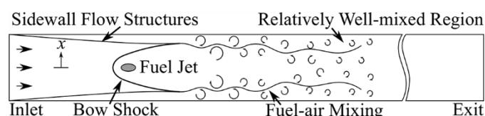
Fig. 6 Top view of the 3D flow structure reconstructed from the 3D PLRS images.
