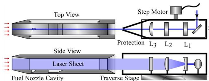
Fig. 3 An optical transformation system in ACT-1.
