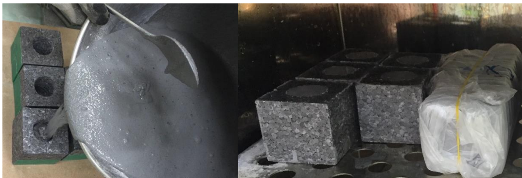
Fig. 4 Pouring and Curing Process
