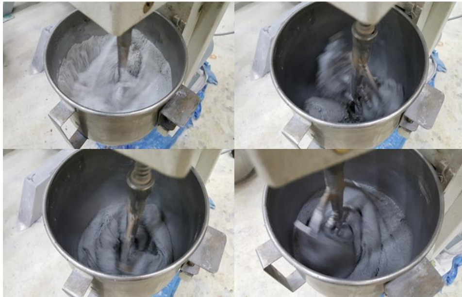
Fig. 3 Mixing Process of UHPC
