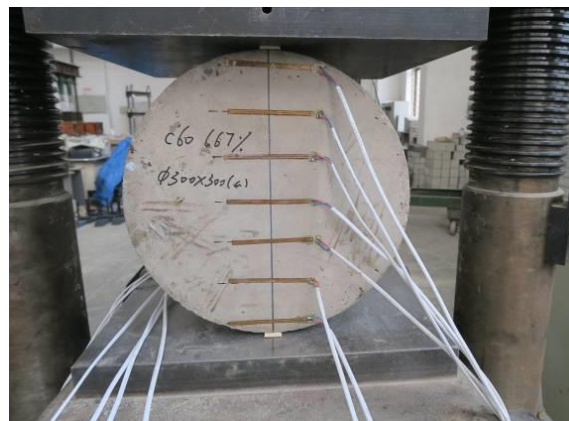
Fig. 2 Specimen with strain gauges
