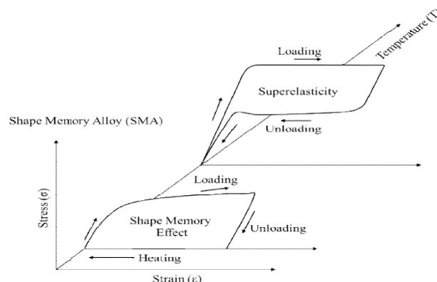
Fig. 1 Superelastic SMA materials
