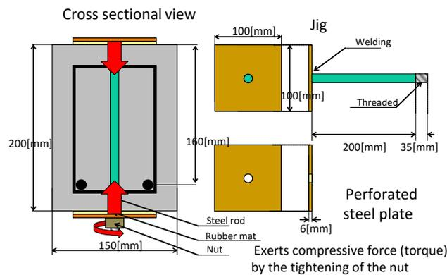
Fig. 2 Experiment outline (cross section and reinforcement method)
