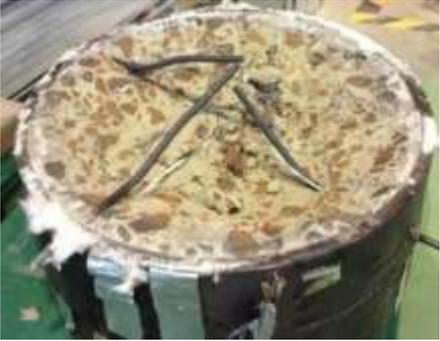
Fig. 10 Spalling after heating test
