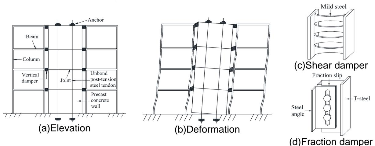
Fig. 1 The concept of frame-SCW system with Vertical dampers
