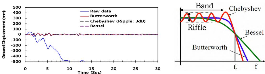
Fig. 2 Comparison of processed data with different filters
