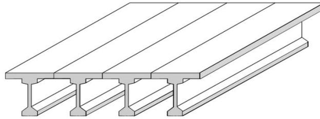
Fig. 1 Decked prestressed concrete girder bridge
