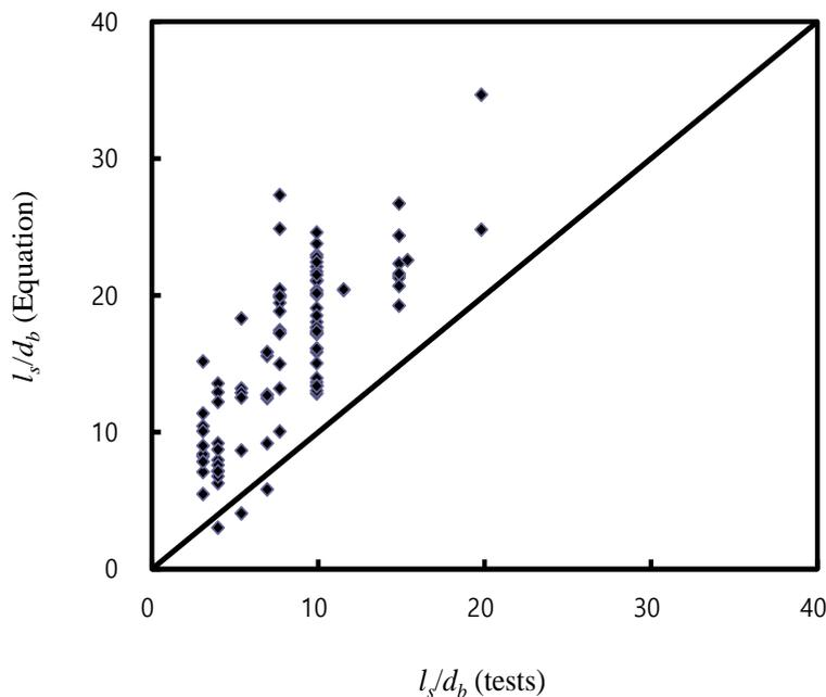
Fig. 3 Calculated  $l_{sd}/d_b$  vs. measured for results reported by Chun et al. (2011)
