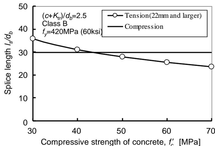
Fig. 1 Comparison of calculated splice lengths with varying concrete compressive strengths. (Chun et al. 2010a)
