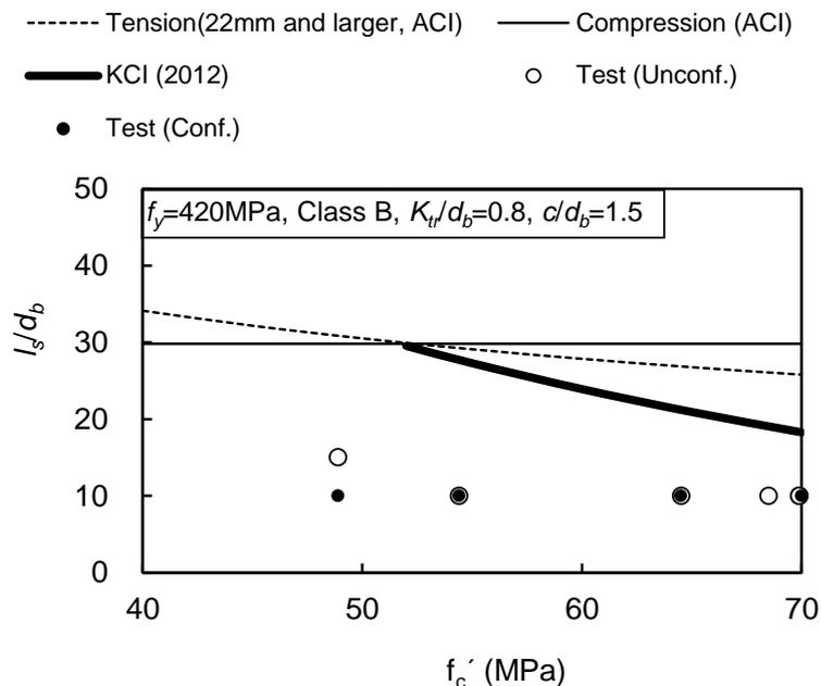
Fig. 4 Splice lengths by ACI 318 (2014) and by KCI (2012) (Chun et al. 2010b)
