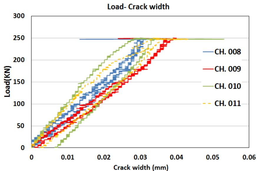
Fig. 6 Load- crack width curve (bottom of joint)
