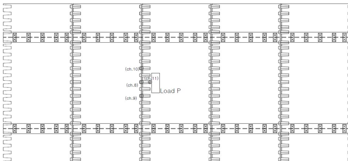
Fig. 4 Static loading setup and crack gauge configuration
