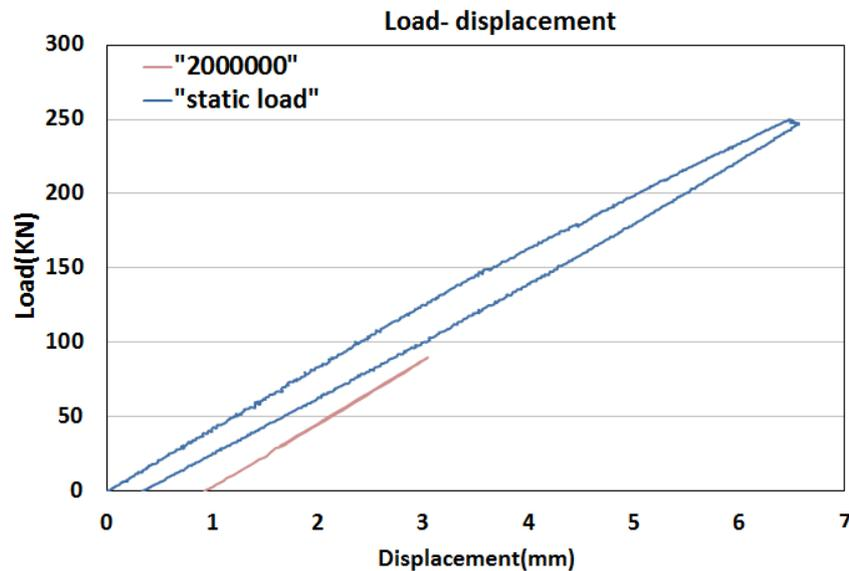
Fig. 5 Load- deflection curve (loading point of specimen)
