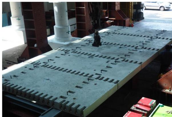
Fig. 1 Load tests of composite bridge using precast concrete deck
