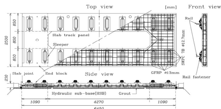
Fig. 1 Precast concrete slab track considered in this paper
