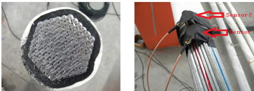
Fig. 5 Cable cross section and sensors layout
