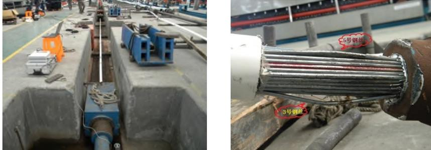
Fig. 6 Cable stretch equipment and breakage wires
