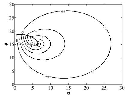
Figure 3. Contour maps of 1<sup>st</sup> mode damping ( $l_1/L=0.02$ ,  $l_2/L=0$ )
