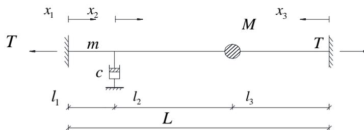
Figure 1. Taut cable with a damper and mass
