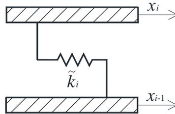
Fig. 3 Shear structure model for the  $i$ -th story
