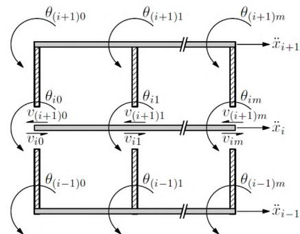
Fig. 2 the  $i$ -th floor substructure
