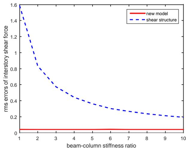
Fig. 6 Relative rmse of interstory shear force for both shear structure model and the new model
