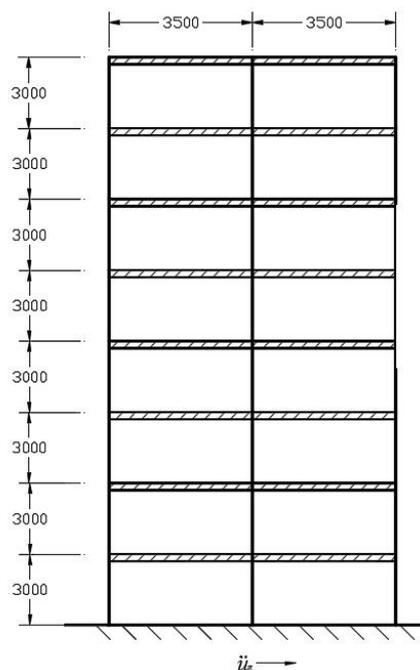
Fig. 5 Numerical example of an 8-story and 2-bay Frame Structure
