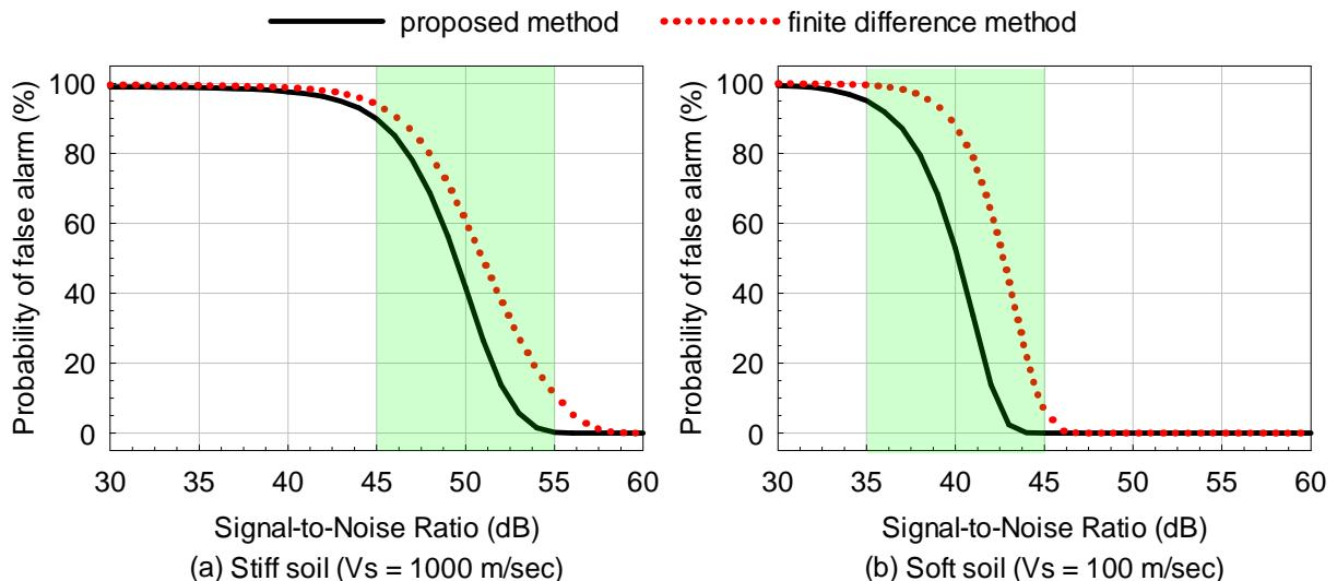
Fig.7 The probability of false alarm against SNR for damage scenario 1
