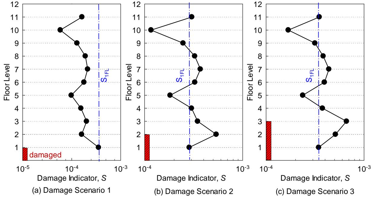
Fig.2 Damage indicator  $S$  using the FRF curvatures from the finite difference method
