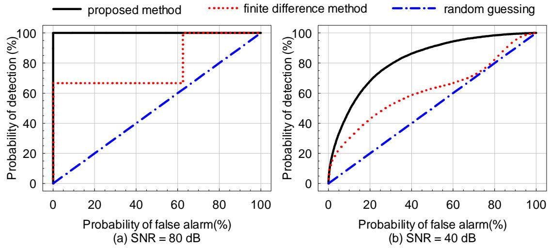
Fig.6 ROC curves for damage scenario 3
