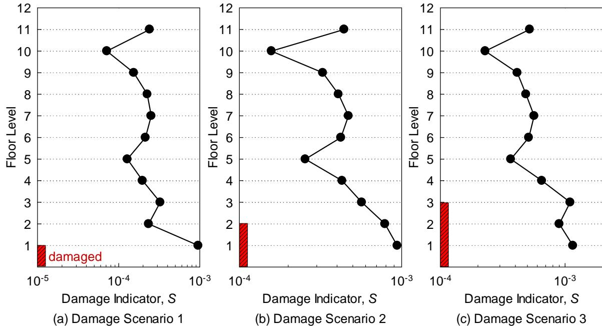
Fig.3 Damage indicator  $S$  using the FRF curvatures from the proposed method
