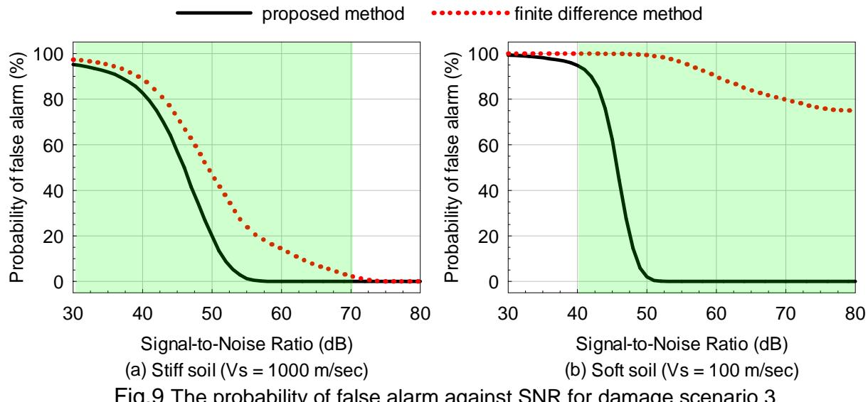
Fig.9 The probability of false alarm against SNR for damage scenario 3
