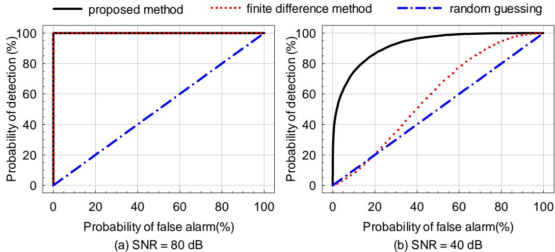
Fig.4 ROC curves for damage scenario 1
