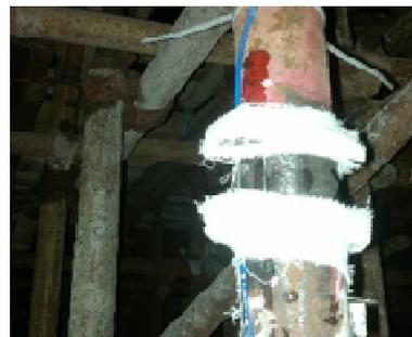
Fig. 4 Protection of FBG sensor in the scaffolding pole
