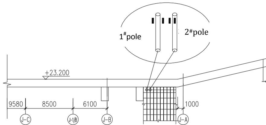
Fig. 2 FBG sensors of scaffolding in+23.200m level
