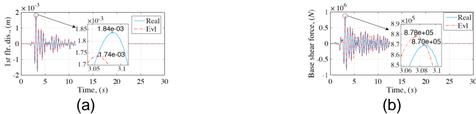
Fig. 2 Comparisons of real and estimated displacement on 1 st floor and base shear
