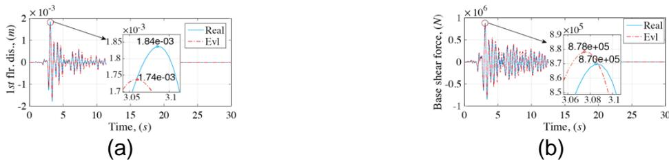
Fig. 2 Comparisons of real and estimated displacement on 1<sup>st</sup> floor and base shear
