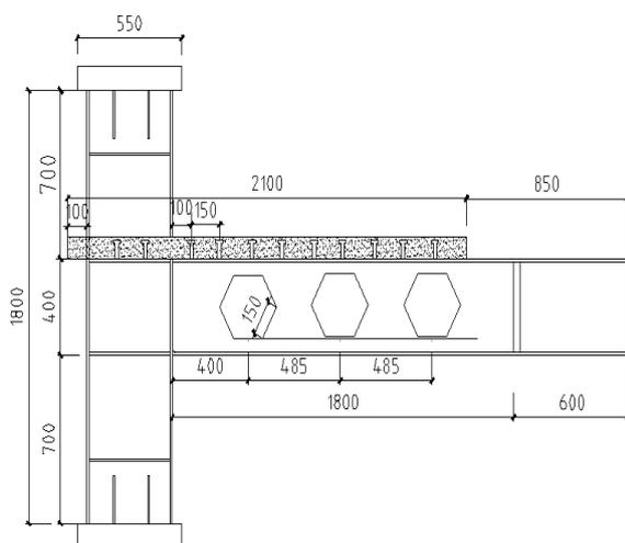
Fig.1 Dimension of specimen
