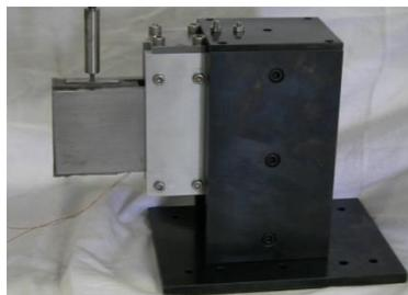
Figure 1 Production of the Prototype Shear Type of MR Damper
