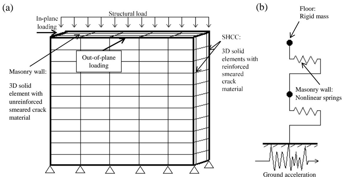
Fig. 1 Analytical models for: (a) Pushover analysis; (b) Dynamic analysis
