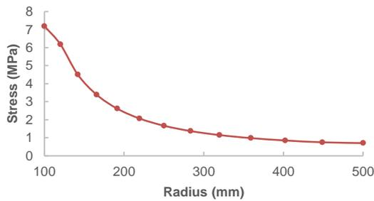
Fig. 6a. Circular stress distribution in pile
