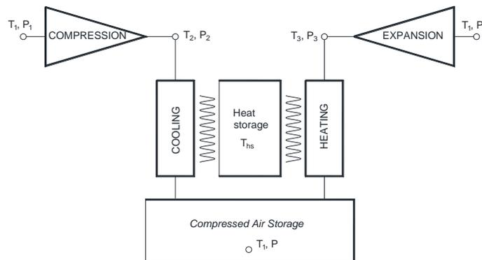
Fig. 1. CAES thermodynamic cycle schematic
