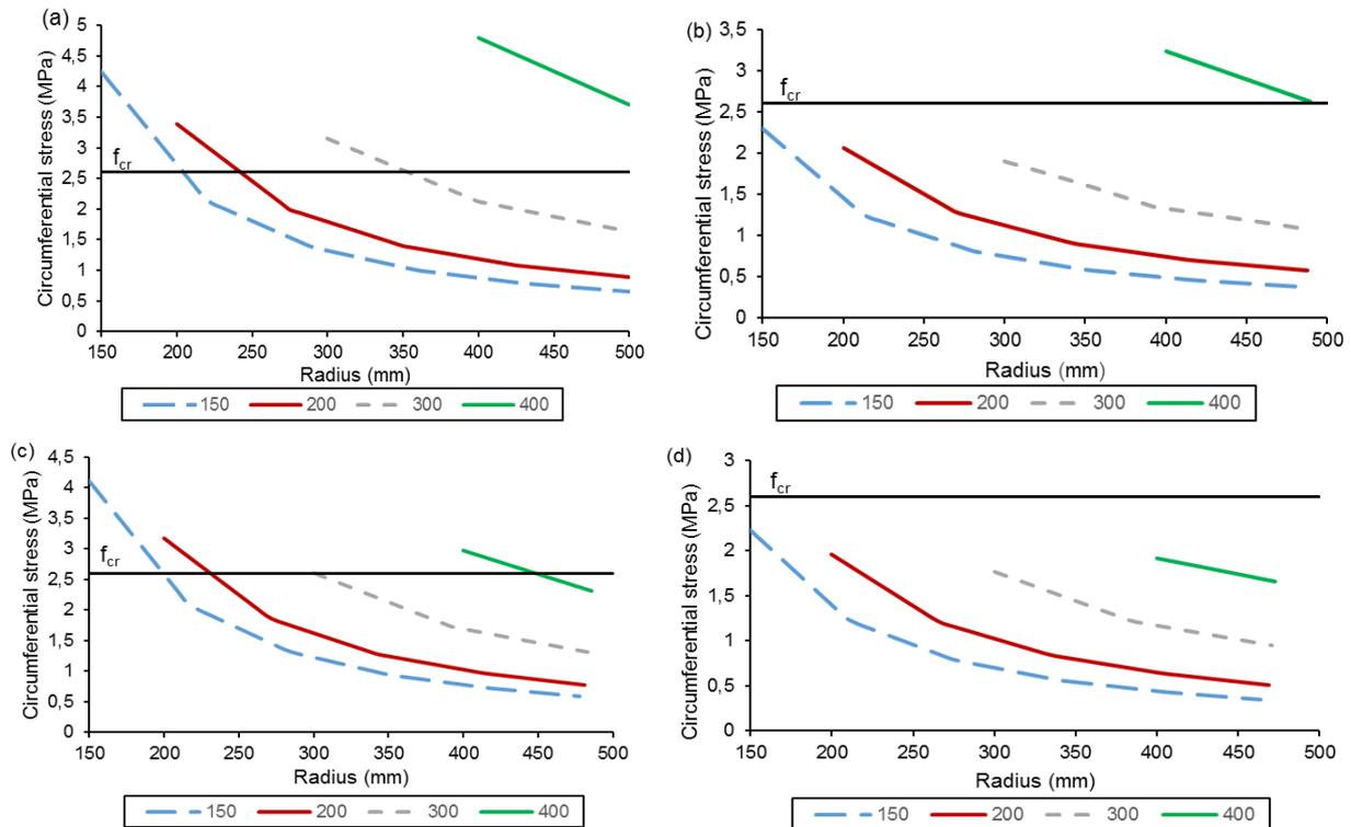
Fig. 4 Circumferential stress of along the radial direction for (a) concrete pile, (b) concrete pile with inner tube, (c) concrete pile with outer tube and (d) concrete pile with double tubes
