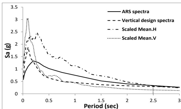
Fig. 2 Scaled spectra for base configuration of multi-span bridge
