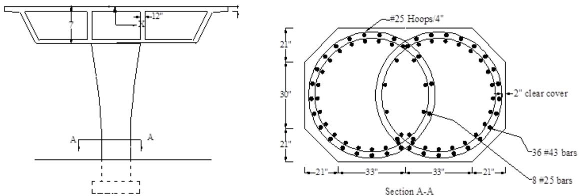
Fig. 1 Elevation view and column details of Amador Creek Bridge
