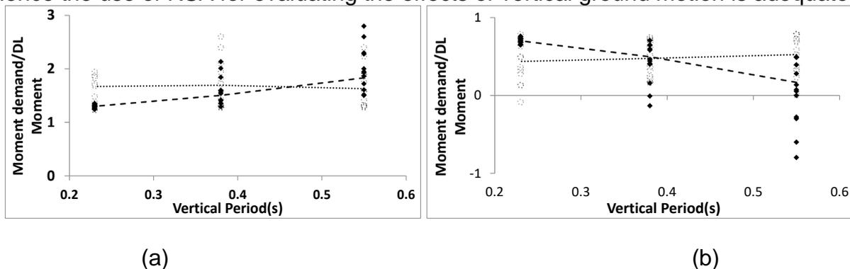
Fig. 3 Comparison of moment demands between RSA and NTH at critical sections for all configurations as a function of vertical periods: (a) Interior mid-span (maximum); (b) Interior mid-span (minimum)
