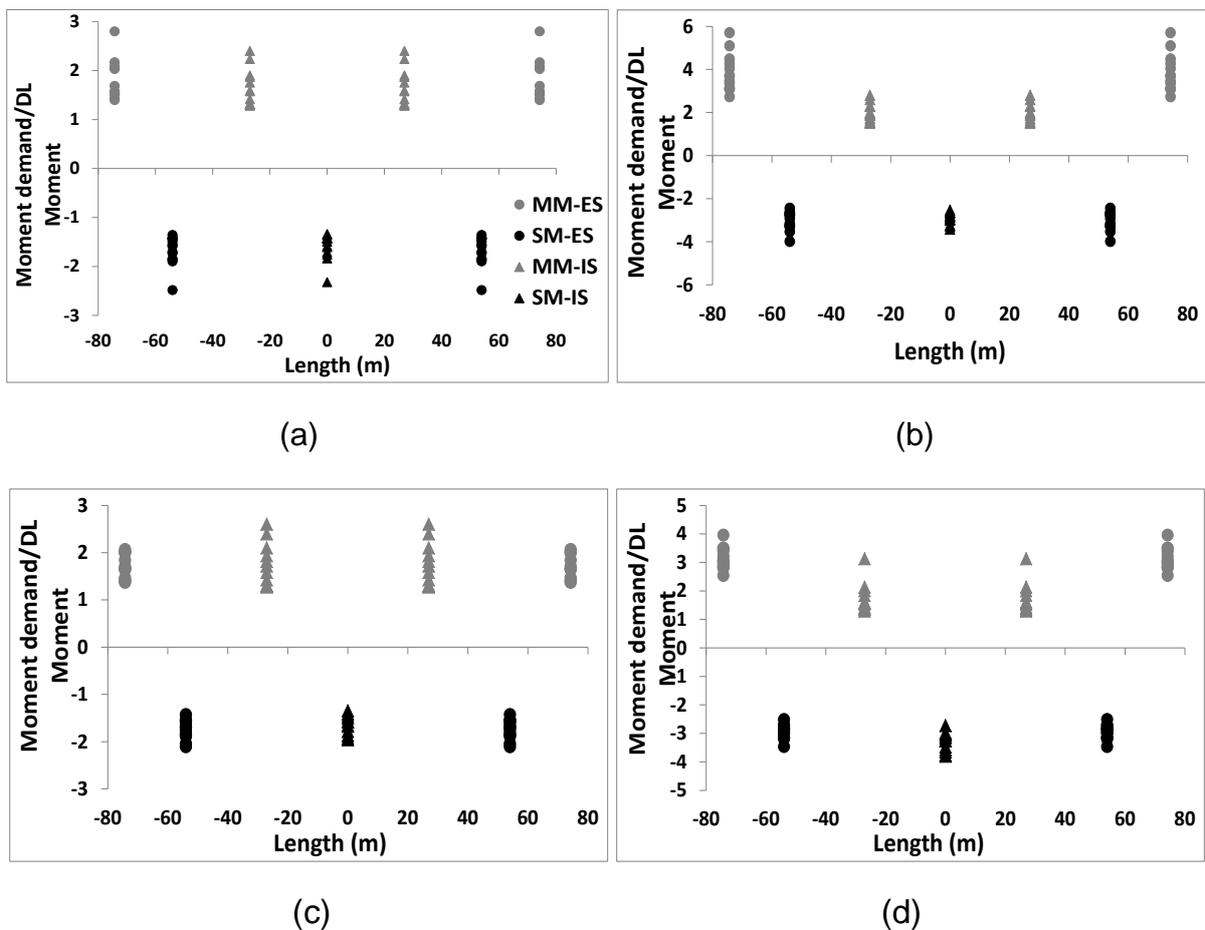
Fig. 4 Comparison of moment demands using NTH and RSA along the deck of Amador Creek Bridge: (a) Configuration 1 – NTH; (b) Configuration 1 – RSA; (c) Configuration 2 – NTH; (d) Configuration 2 – RSA.
