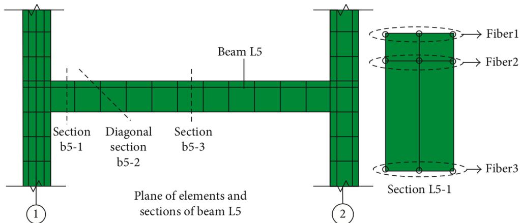
**Fig.4** The analysis objects of member-level, section-level and material-level
