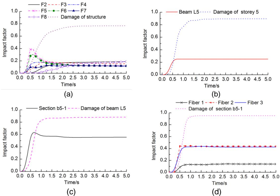
**Fig.3** Damage correlations between different levels. (a) Storey-level to structure-level. (b) Member-level to storey-level. (c) Section-level to member-level. (d) Material-level to section-level.
