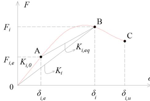
Fig.2 Generalized force-deformation relationship (Jianguang 2016)
