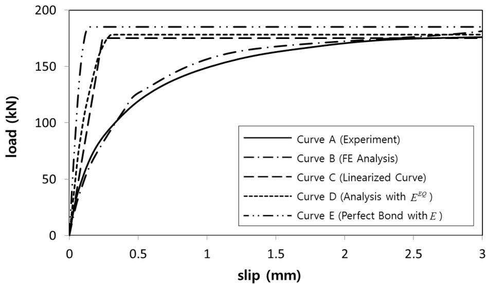
Fig. 1 Load-slip curve of Push-out test
