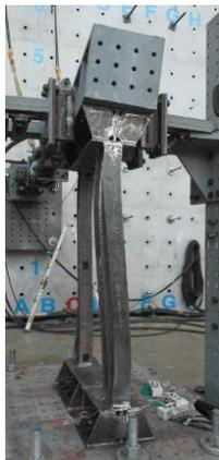
(a) Deformed shape at end of test
