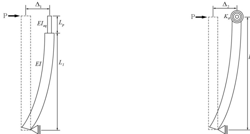
(a) RC beam with  $EI_{eq}$  (b) RC beam with  $K_\theta$
